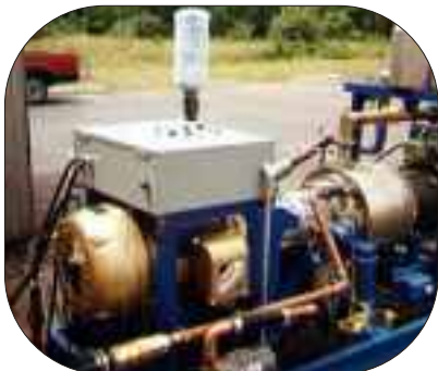
STM's BioStirling™ system is one example of the modular power units being developed under this initiative.
